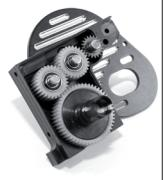
Once you have the layshaft spacing tuned correctly. Place all the gears into place. The gears will all sit at the same height.
