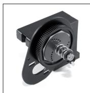
Using the 2 long screws and 2x 1mm washers screw the gearbox case together ensuring you take your time and don't cross thread the motor plate.
